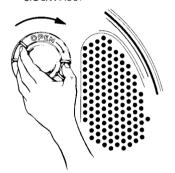
2. Remove the light bulb by turning it counterclockwise.
